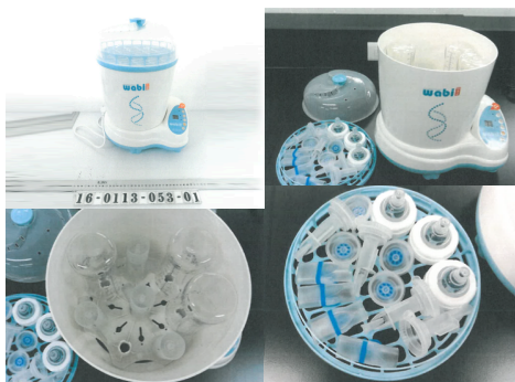
Figure 2. showcasing sample items placed randomly inside the chamber with the given instruction not to block the air circulation between the samples.
